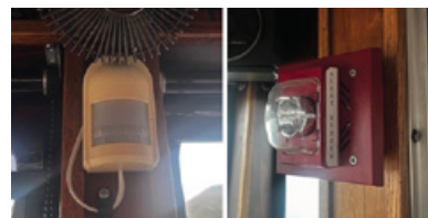
Left to right: Cindy B pilothouse alerter system motion detector (one of two on board) and strobe light with audible alarm.
