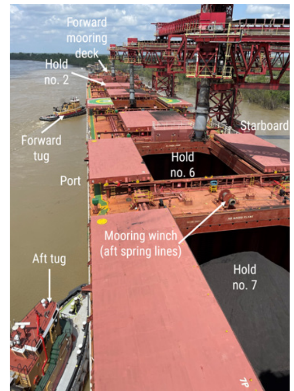
The two tugs on the Sirocco 's port side on March 26 at 1314. BACKGROUND SOURCE: OLDENDORFF PORT CAPTAIN.
