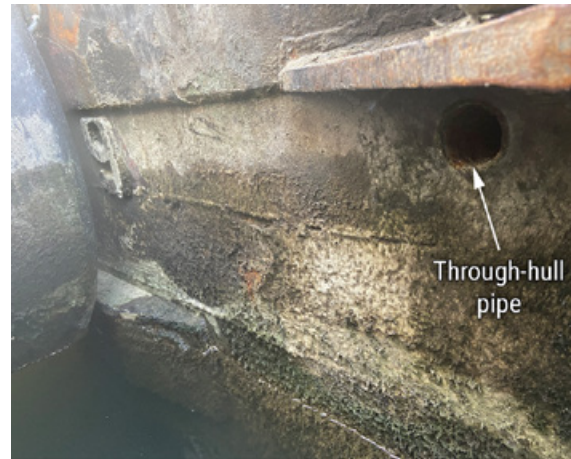
Joanne Marie cofferdam discharge system (facing aft). BACKGROUND SOURCE: COAST GUARD.
