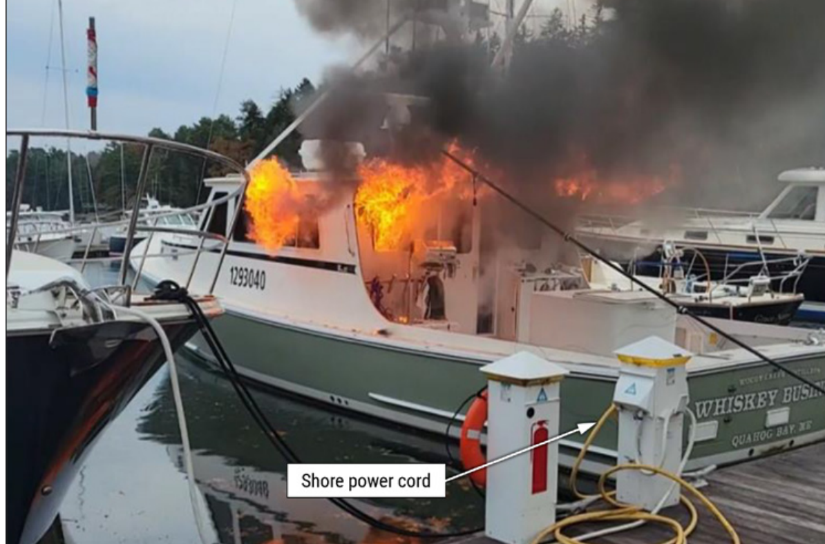
Fire aboard the Whiskey Business , about 0918 on November 5, 2024. The shore power cord had been connected from the shore power pedestal to the boat. BACKGROUND SOURCE: MARK LENZI.
