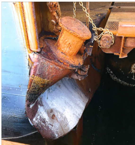
San Juan-JAX Bridge's damaged port quarter.
