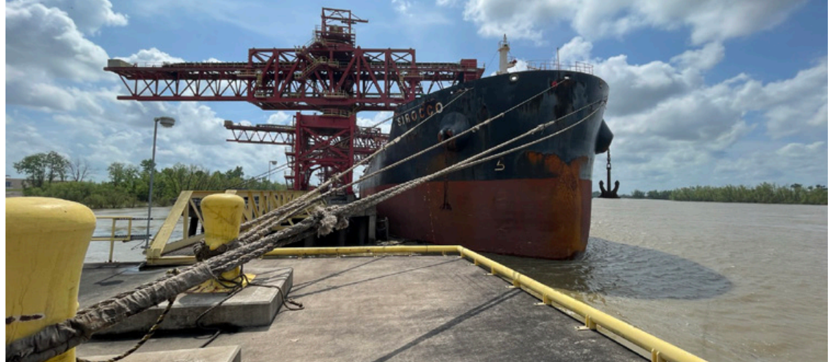
The forward mooring arrangement of the Sirocco at the Convent Marine Terminal dock at 1227 on March 26, 2023. SOURCE: OLDENDORFF PORT CAPTAIN.
