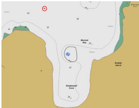
ENC US4AK5PM, for the area near Shakmanof Cove, as viewed by investigators using an equivalent ECS. The asterisk symbol for the rock in the area of the grounding is indicated by a red circle. BACKGROUND SOURCE: NOAA ENC AS VIEWED ON ROSE POINT ECS.
