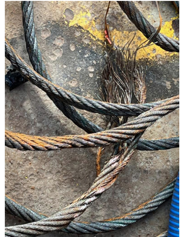
Parted wire after the breakaway.
