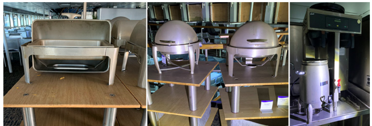
Left to right: Spirit of Boston chafing dishes (with the chafing fuel heating canisters removed) in passenger areas on deck 2 and deck 3 after the fire. Exemplar coffee maker and dispenser used aboard Spirit of Boston with the chafing fuel heating canisters removed from under the dispenser.
