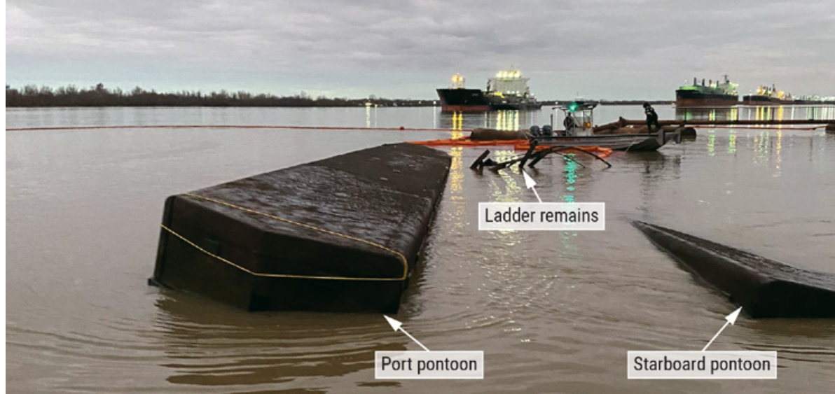
The overturned hull of the WB Wood with its pontoons downside up, the morning after the capsizing.
