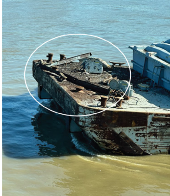
Left to right: The damage to barge ACBL2549 after the contact (circled), and the damage to the Port of West Memphis dock (circled). SOURCE: COAST GUARD.
