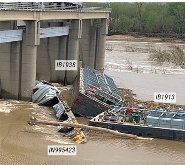
Barges IN995423 and IB1938 against the lower dam gates. IB1913 is receiving methanol from IB1938 through a cargo transfer hose.
