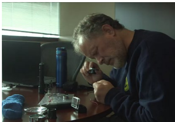
Figure 10. Matthew Fox, chief technical advisor, Materials Laboratory, examines the wires and connectors of a Rutan VariEze that sustained substantial damage during landing in Columbia, California on September 5, 2022. The pilot was fatally injured.
