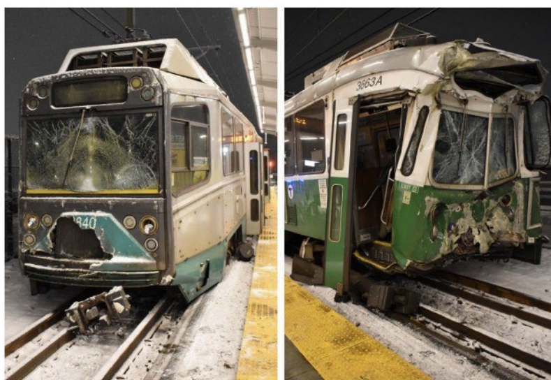
Figure 8. The Massachusetts Bay Transportation Authority (MBTA) light rail train collided with a stationary MBTA light rail train damaging four cars and derailing one car on each train on February 9, 2025, in Somerville, MA.
