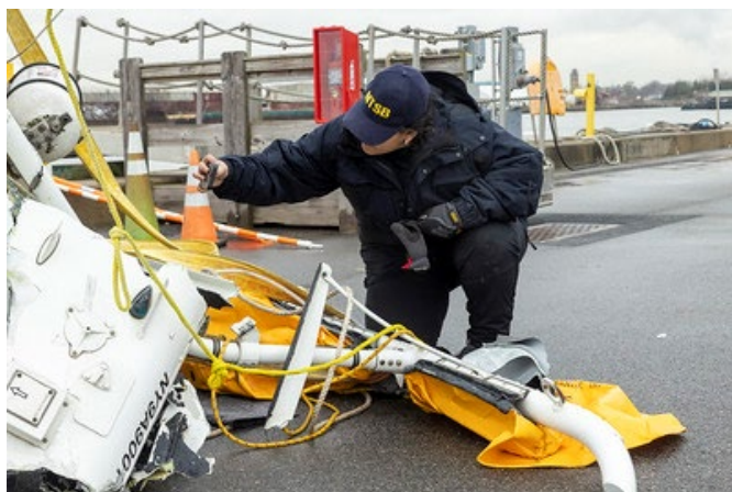
Figure 5. An NTSB aerospace engineer investigating the wreckage recovered from the Bell 206 L-4 helicopter that crashed into the Hudson River on April 10, 2025, near Jersey City, New Jersey. Based on a witness, the helicopter was in cruise flight when an inflight breakup occurred, resulting in a separation of the main rotor, tail rotor, and tail boom from the main fuselage.
