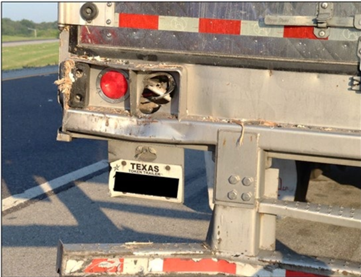
Figure 13. Damage to the left rear of the Mack vehicle's semitrailer. (Source: ISP)
