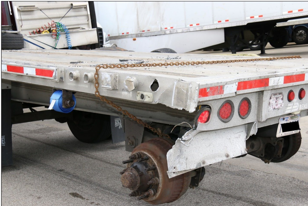
Figure 12. Damage to the left rear of the Kenworth vehicle's semitrailer.
