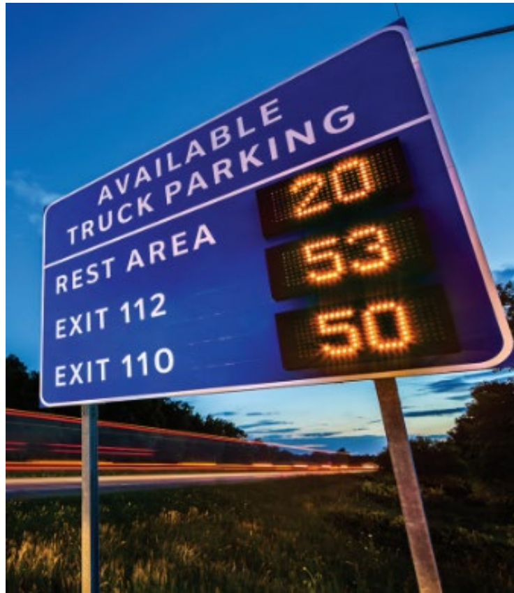
Figure 19. Photo of an exemplar variable message sign that shows availability of truck parking. (Source: National Coalition on Truck Parking)
