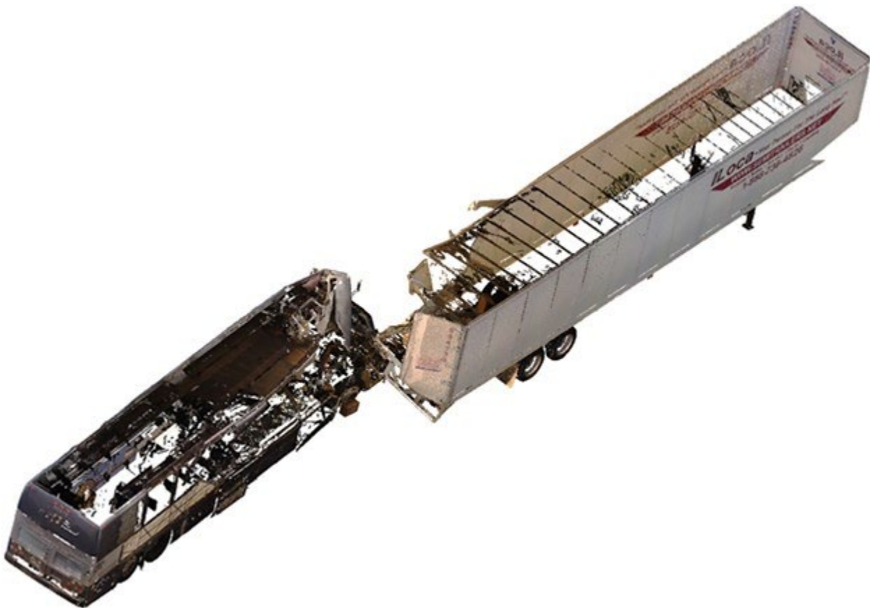
Figure 17. Illustration of vehicle impact orientation, using 3-dimensional scans.
