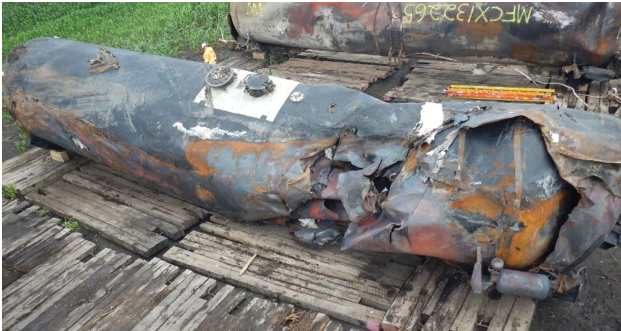
Figure 21. Shell tear, torn jacket, and missing thermal blanket on CTCX732476.
