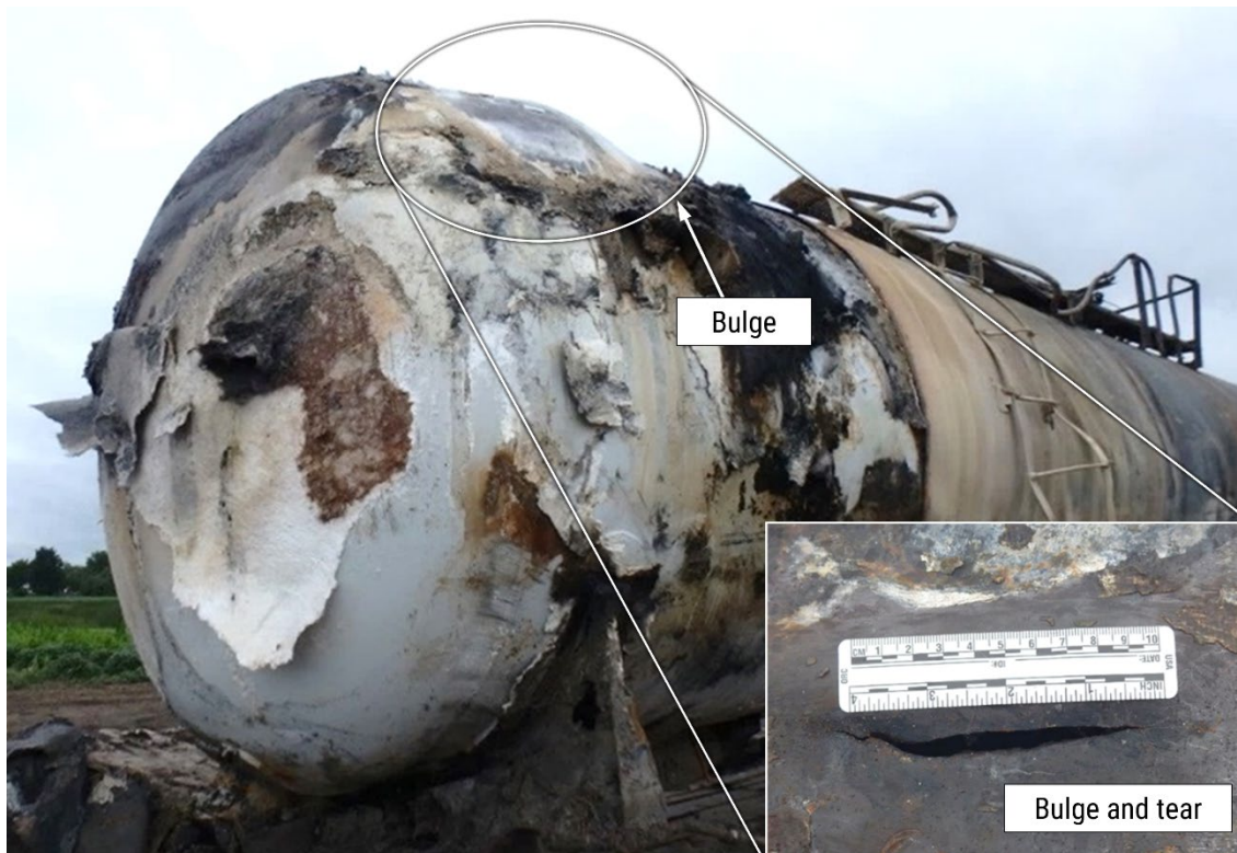
Figure 16. Bulge in tank car (59) SHQX10805 ( upper left ) and thermal tear ( inset ).
