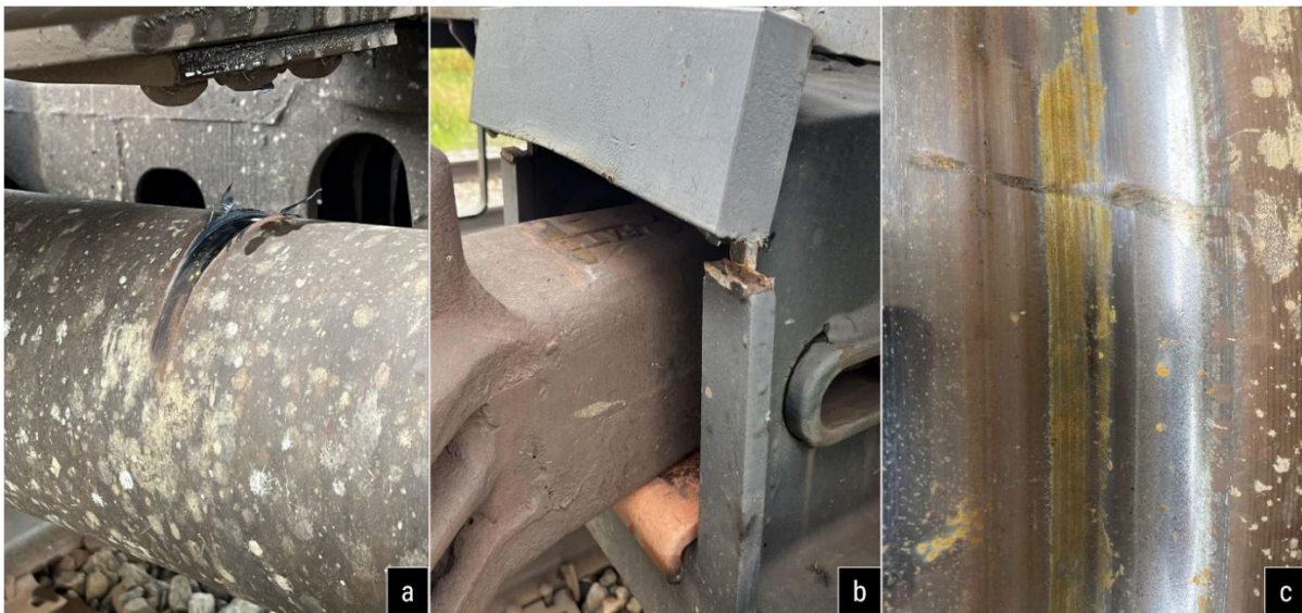
Figure 10. Damage to non-derailed equipment: (a) axle contact with draft sill, (39) TILX500825; (b) damaged buffer casting, (46) PROX43474; and (c) broken-rail witness mark on wheel, (41) SHQX10687.
