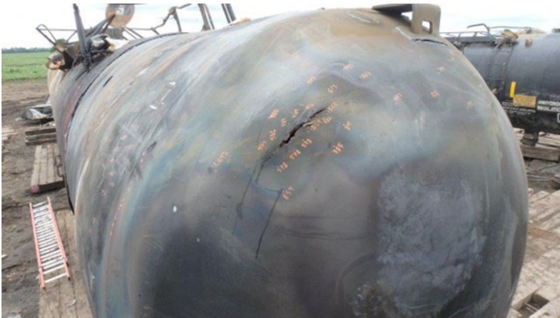
Figure 14. B-end head bulge and tear.
