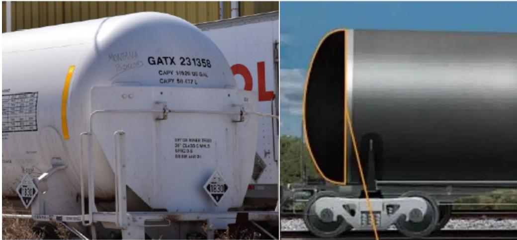
Figure 31. An example of a half-height head shield ( left ) and a full-height head shield ( right ), which is typically built into the tank shell. (Source: AAR.)
