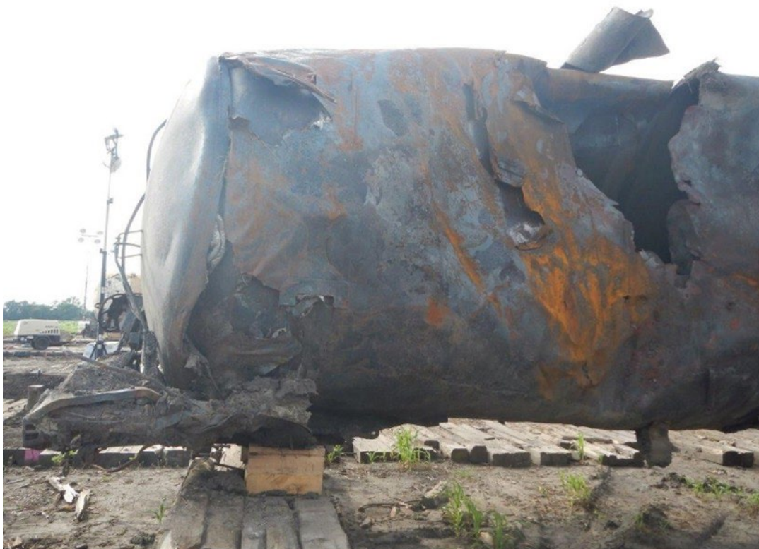
Figure 19. Shell fracture on tank car (61) TILX355610.
